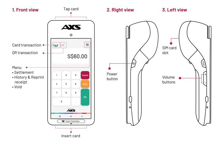
Press and hold the Power (3) button to turn on your device.
